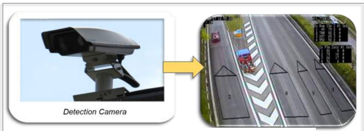
Figure 3. Detection Cameras and Virtual Loops of EMAS and EA Systems
