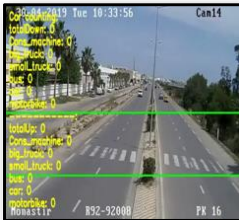
Camera AI for road traffic counting and speed
