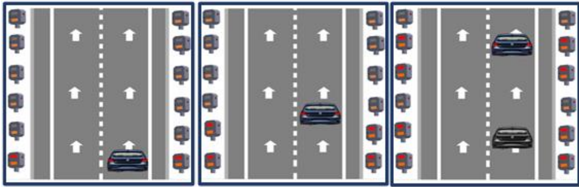
Figure 6– Project of beacons in low visibility conditions. A-8 Motorway. Alto del Fiuoco (Lugo). Spain
